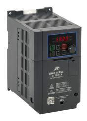
IronHorse ACG series AC general purpose drive, enclosed, 230 VAC, 3hp with 3-phase input, 1-1/2hp with 1-phase input, SVC or V/Hz mode, B frame, RS-485, Modbus, 100kA SCCR. Optional EtherNet/IP and Modbus TCP card available.
