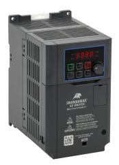
IronHorse ACG series AC general purpose drive, enclosed, 230 VAC, 2hp with 3-phase input, 1hp with 1-phase input, SVC or V/Hz mode, B frame, RS-485, Modbus, 100kA SCCR. Optional EtherNet/IP and Modbus TCP card available.
