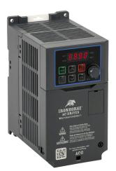
IronHorse ACG series AC general purpose drive, enclosed, 230 VAC, 1hp with 3-phase input, 1/2hp with 1-phase input, SVC or V/Hz mode, A frame, RS-485, Modbus, 100kA SCCR. Optional EtherNet/IP and Modbus TCP card available.
