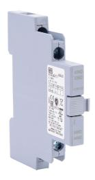
WEG Electric field installable auxiliary contact, left side mount, (2) N.O. contact(s), 6A @ 120 VAC/0.55A @ 120 VDC, screw terminal. For use with MPW40 and MPW80 series manual motor protectors.
