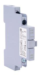
WEG Electric field installable auxiliary contact, left side mount, (2) N.C. contact(s), 6A @ 120 VAC/0.55A @ 120 VDC, screw terminal. For use with MPW40 and MPW80 series manual motor protectors.
