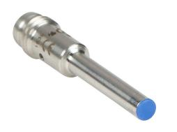
Micro Detectors inductive proximity sensor, tubular, 4mm diameter x 38.5mm body, stainless steel housing, PNP, N.C. output, 1.5mm sensing distance, flush, 7 kHz switching frequency, IP67, 3-pin M8 quick-disconnect.
