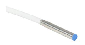
Micro Detectors inductive proximity sensor, tubular, 4mm diameter x 30.2mm body, stainless steel housing, PNP, N.C. output, 1.5mm sensing distance, flush, 7 kHz switching frequency, IP67, pigtail.
