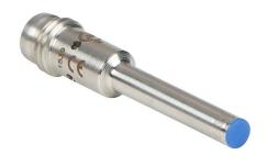
Micro Detectors inductive proximity sensor, tubular, 4mm diameter x 38.5mm body, stainless steel housing, PNP, N.C. output, 0.8mm sensing distance, flush, 7 kHz switching frequency, IP67, 3-pin M8 quick-disconnect.
