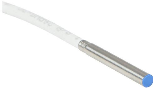
Micro Detectors inductive proximity sensor, tubular, 4mm diameter x 30.2mm body, stainless steel housing, PNP, N.C. output, 0.8mm sensing distance, flush, 7 kHz switching frequency, IP67, pigtail.
