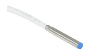
Micro Detectors inductive proximity sensor, tubular, 4mm diameter x 30.2mm body, stainless steel housing, PNP, N.C. output, 0.8mm sensing distance, flush, 7 kHz switching frequency, IP67, pigtail.
