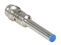
Micro Detectors inductive proximity sensor, tubular, 4mm diameter x 38.5mm body, stainless steel housing, NPN, N.C. output, 1.5mm sensing distance, flush, 7 kHz switching frequency, IP67, 3-pin M8 quick-disconnect.
