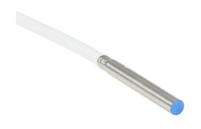
Micro Detectors inductive proximity sensor, tubular, 4mm diameter x 30.2mm body, stainless steel housing, NPN, N.C. output, 1.5mm sensing distance, flush, 7 kHz switching frequency, IP67, pigtail.
