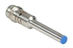
Micro Detectors inductive proximity sensor, tubular, 4mm diameter x 38.5mm body, stainless steel housing, NPN, N.C. output, 0.8mm sensing distance, flush, 7 kHz switching frequency, IP67, 3-pin M8 quick-disconnect.
