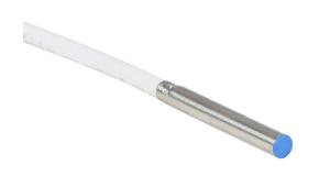
Micro Detectors inductive proximity sensor, tubular, 4mm diameter x 30.2mm body, stainless steel housing, NPN, N.C. output, 0.8mm sensing distance, flush, 7 kHz switching frequency, IP67, pigtail.
