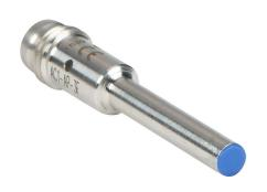
Micro Detectors inductive proximity sensor, tubular, 4mm diameter x 38.5mm body, stainless steel housing, PNP, N.O. output, 1.5mm sensing distance, flush, 7 kHz switching frequency, IP67, 3-pin M8 quick-disconnect.
