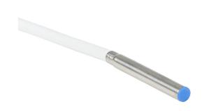
Micro Detectors inductive proximity sensor, tubular, 4mm diameter x 30.2mm body, stainless steel housing, PNP, N.O. output, 1.5mm sensing distance, flush, 7 kHz switching frequency, IP67, pigtail.
