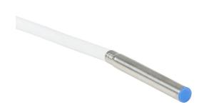
Micro Detectors inductive proximity sensor, tubular, 4mm diameter x 30.2mm body, stainless steel housing, PNP, N.O. output, 1.5mm sensing distance, flush, 7 kHz switching frequency, IP67, pigtail.
