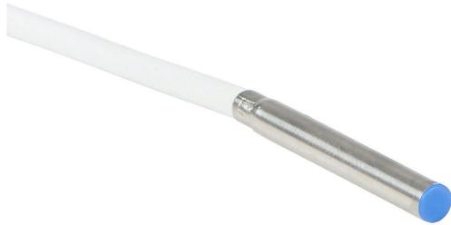
Micro Detectors inductive proximity sensor, tubular, 4mm diameter x 30.2mm body, stainless steel housing, PNP, N.O. output, 1.5mm sensing distance, flush, 7 kHz switching frequency, IP67, pigtail.
