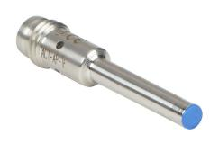
Micro Detectors inductive proximity sensor, tubular, 4mm diameter x 38.5mm body, stainless steel housing, PNP, N.O. output, 0.8mm sensing distance, flush, 7 kHz switching frequency, IP67, 3-pin M8 quick-disconnect.
