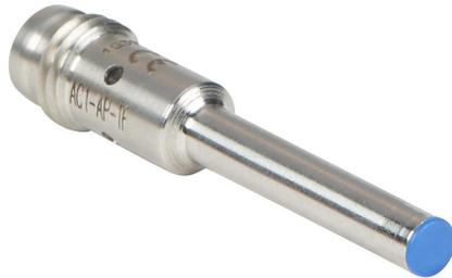
Micro Detectors inductive proximity sensor, tubular, 4mm diameter x 38.5mm body, stainless steel housing, PNP, N.O. output, 0.8mm sensing distance, flush, 7 kHz switching frequency, IP67, 3-pin M8 quick-disconnect.
