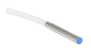
Micro Detectors inductive proximity sensor, tubular, 4mm diameter x 30.2mm body, stainless steel housing, NPN, N.O. output, 1.5mm sensing distance, flush, 7 kHz switching frequency, IP67, pigtail.
