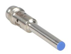
Micro Detectors inductive proximity sensor, tubular, 4mm diameter x 38.5mm body, stainless steel housing, NPN, N.O. output, 0.8mm sensing distance, flush, 7 kHz switching frequency, IP67, 3-pin M8 quick-disconnect.
