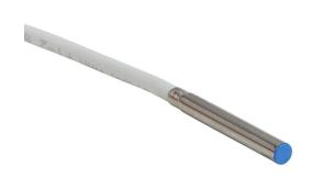
Micro Detectors inductive proximity sensor, tubular, 4mm diameter x 30.2mm body, stainless steel housing, NPN, N.O. output, 0.8mm sensing distance, flush, 7 kHz switching frequency, IP67, pigtail.
