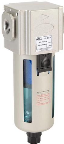
NITRA pneumatic filter, coalescing, 1/2in female NPT inlet(s), 1/2in female NPT outlet(s), manual/semi-automatic drain, nylon bowl, metal bowl guard. For use with Ax-44 series air prep components.
