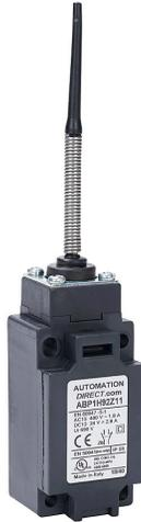
AutomationDirect IEC limit switch, 360 degree stainless steel spring with polyamide tip, 90-degree adjustable head, (1) N.O./ (1) N.C. contact(s), snap action, 30mm hole spacing, plastic, (1) PG13.5 cable entry.
