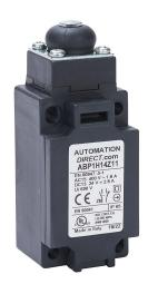
AutomationDirect IEC limit switch, metal plunger, 90-degree adjustable head, (1) N.O./(1) N.C. contact(s), snap action, 30mm hole spacing, plastic, (1) PG13.5 cable entry.
