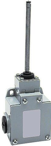
AutomationDirect IEC limit switch, 360 degree stainless steel spring, 90-degree adjustable head, (1) N.O./ (1) N.C. contact(s), snap action, 40mm hole spacing, aluminum, (3) 1/2in NPT cable entries.
