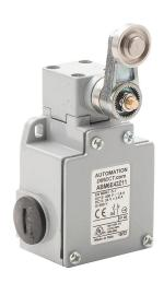
AutomationDirect IEC limit switch, side rotary lever with stainless steel roller, 90-degree adjustable head, (1) N.O./(1) N.C. contact(s), snap action, 40mm hole spacing, aluminum, (3) 1/2in NPT cable entries.
