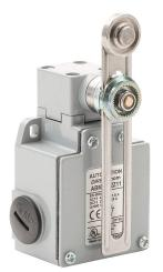
AutomationDirect IEC limit switch, side rotary adjustable lever with stainless steel roller, 90-degree adjustable head, (1) N.O./(1) N.C. contact(s), snap action, 40mm hole spacing, aluminum, (3) PG13.5 cable entries.
