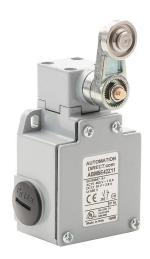
AutomationDirect IEC limit switch, side rotary lever with stainless steel roller, 90-degree adjustable head, (1) N.O./(1) N.C. contact(s), snap action, 40mm hole spacing, aluminum, (3) PG13.5 cable entries.
