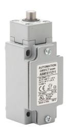
AutomationDirect IEC limit switch, stainless steel plunger, 90-degree adjustable head, (1) N.O./(1) N.C. contact(s), snap action, 30mm hole spacing, aluminum, (1) PG13.5 cable entry.
