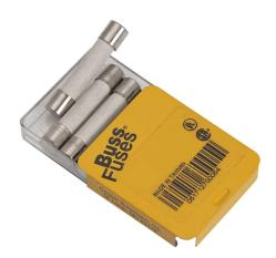
Bussmann fuse, ABC series, small dimension, fast-acting, 6A, 250 VAC, ceramic tube. Package of 5. Supplemental, electronic protection applications. Manufacturer part number: ABC-6-R.
