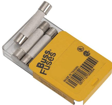
Bussmann fuse, ABC series, small dimension, fast-acting, 5A, 250 VAC, ceramic tube. Package of 5. Supplemental, electronic protection applications. Manufacturer part number: ABC-5-R.
