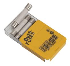
Bussmann fuse, ABC series, small dimension, fast-acting, 3A, 250 VAC, ceramic tube. Package of 5. Supplemental, electronic protection applications. Manufacturer part number: ABC-3-R.
