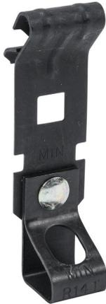
Minerallac z-purlin rod hanger, package of 100. For use with 1/16 to 1/4in z-purlin and 1/4-20 UNC threaded rod.
