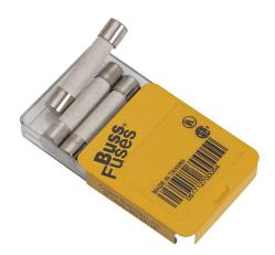
Bussmann fuse, ABC series, small dimension, fast-acting, 10A, 250 VAC, ceramic tube. Package of 5. Supplemental, electronic protection applications. Manufacturer part number: ABC-10-R.
