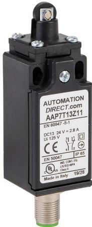
AutomationDirect IEC limit switch, galvanized steel plunger with polyamide plastic roller, 90-degree adjustable head, (1) N.O./ (1) N.C. contact(s), snap action, 20-22mm hole spacing, plastic, (1) 5-pin M12 quick-disconnect.
