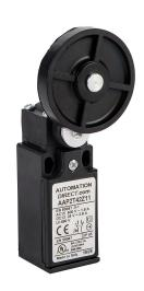
AutomationDirect IEC limit switch, side rotary lever with 50mm rubber roller, 90-degree adjustable head, (1) N.O./(1) N.C. contact(s), snap action, 20-22mm hole spacing, plastic, (1) PG11 cable entry with 1/2in NPT adapter.
