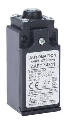
AutomationDirect IEC limit switch, galvanized steel plunger, 90-degree adjustable head, (1) N.O./(1) N.C. contact(s), snap action, 20-22mm hole spacing, plastic, (1) PG11 cable entry with 1/2in NPT adapter.
