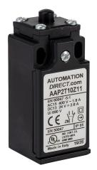
AutomationDirect IEC limit switch, plastic plunger, 90-degree adjustable head, (1) N.O./(1) N.C. contact(s), snap action, 20-22mm hole spacing, plastic, (1) PG11 cable entry with 1/2in NPT adapter.
