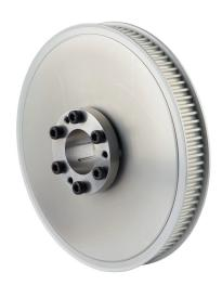
Sung-Il Machinery timing pulley, aluminum, 5mm 5M pitch, 96 tooth, 6.015in pitch diameter, 1-1/8in bore, no hub with flanges. For use with 15mm wide belt. QD bushing included.
