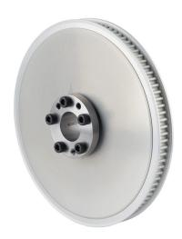
Sung-Il Machinery timing pulley, aluminum, 5mm 5M pitch, 96 tooth, 6.015in pitch diameter, 7/8in bore, no hub with flanges. For use with 9mm wide belt. QD bushing included.
