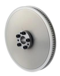
Sung-Il Machinery timing pulley, aluminum, 5mm 5M pitch, 96 tooth, 6.015in pitch diameter, 3/4in bore, no hub with flanges. For use with 9mm wide belt. QD bushing included.
