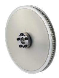
Sung-Il Machinery timing pulley, aluminum, 5mm 5M pitch, 96 tooth, 6.015in pitch diameter, 5/8in bore, no hub with flanges. For use with 9mm wide belt. QD bushing included.
