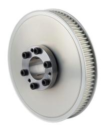
Sung-Il Machinery timing pulley, aluminum, 5mm 5M pitch, 84 tooth, 5.263in pitch diameter, 1-1/8in bore, no hub with flanges. For use with 15mm wide belt. QD bushing included.
