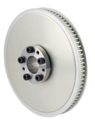
Sung-Il Machinery timing pulley, aluminum, 5mm 5M pitch, 84 tooth, 5.263in pitch diameter, 7/8in bore, no hub with flanges. For use with 9mm wide belt. QD bushing included.
