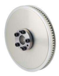
Sung-Il Machinery timing pulley, aluminum, 5mm 5M pitch, 84 tooth, 5.263in pitch diameter, 3/4in bore, no hub with flanges. For use with 9mm wide belt. QD bushing included.
