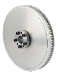
Sung-Il Machinery timing pulley, aluminum, 5mm 5M pitch, 84 tooth, 5.263in pitch diameter, 5/8in bore, no hub with flanges. For use with 9mm wide belt. QD bushing included.
