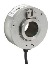
Lika Electronic A80 series incremental (quadrature) rotary encoder, medium duty, 5-30 VDC, radial exit, universal (line driver or NPN/PNP open collector) output, 1024 ppr, multiple shafts (5/8in - 30mm), 80mm diameter body, IP64, 6.5ft/2m cable length, pigtail.
