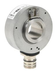
Lika Electronic A80 series incremental (quadrature) rotary encoder, medium duty, 5-30 VDC, radial exit, universal (line driver or NPN/PNP open collector) output, 1024 ppr, multiple shafts (5/8in - 30mm), 80mm diameter body, IP64, M23 male.
