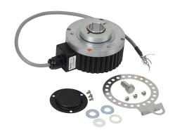
Marathon incremental (quadrature) rotary encoder kit, 5-26 VDC, line driver (differential) output, 1024 ppr, IP67. For use with Marathon Blue Max TEBC encoder motors. Mounting hardware included. Dynapar HS38 encoder.
