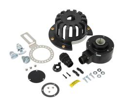
Marathon incremental (quadrature) rotary encoder kit, 5-26 VDC, line driver (differential) output, 1024 ppr, IP67. For use with Marathon Blue Max TEFC encoder motors. Mounting hardware included. Dynapar HS35 encoder.
