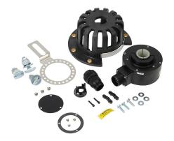
Marathon incremental (quadrature) rotary encoder kit, 5-26 VDC, line driver (differential) output, 1024 ppr, IP67. For use with Marathon Blue Max TEFC encoder motors. Mounting hardware included. Dynapar HS35 encoder.
