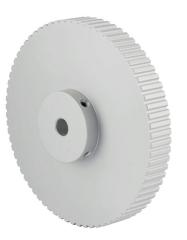
Sung-Il Machinery timing pulley, aluminum, 1/5in XL pitch, 72 tooth, 4.584in pitch diameter, 3/8in bore, hub without flanges. For use with 3/8in wide belt.
