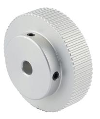
Sung-Il Machinery timing pulley, aluminum, 0.08in MXL pitch, 72 tooth, 1.833in pitch diameter, 1/4in bore, hub without flanges. For use with 1/4in wide belt.
